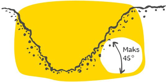
*With intersecting trenches in disturbed ground, the trench walls must have a maximum angle of 45°, even if the trench depth is less than 2 m.*
