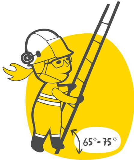
*Ladders must be secured at the top or bottom, or held by another person. Inclined ladders must be leant at an angle of between 65° and 75°.*
