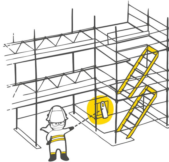
***Scaffolding must have safe, convenient and appropriate access, preferably with a separate external stair tower. Only personnel who have received appropriate training can assemble, modify and disassemble scaffolding/travelling scaffolding.***
