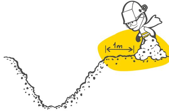
*Excavated material must always be placed at least one metre from the edge in order to avoid an increased risk of collapse.*
