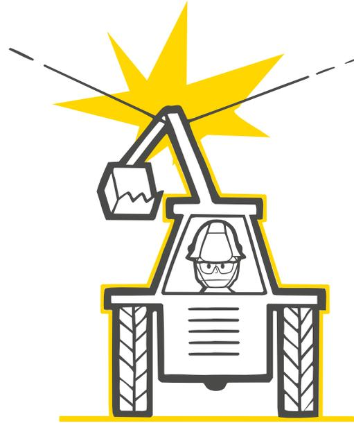
*If a flashover occurs, no one must touch the machine. The operator must remain seated in the driver's seat until the line has been disconnected and the owner of the high voltage installation has given the okay signal for evacuation. Most high voltage installations have automatic re-engagement, i.e. the line will automatically try to restore voltage following a short circuit. Machines must not be touched or moved until qualified personnel with high voltage expertise are present.*
